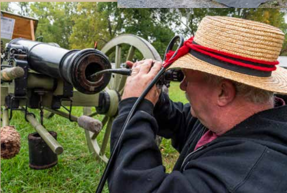
Artillery pieces must be fully inspected prior to being fired in their first N-SSA event, and then re-inspected every five years or whenever ownership of the piece changes. Here, National Artillery Officer Rob West uses a scope to inspect the breech and vent of a 6-pounder gun. (Ericka Curley)
