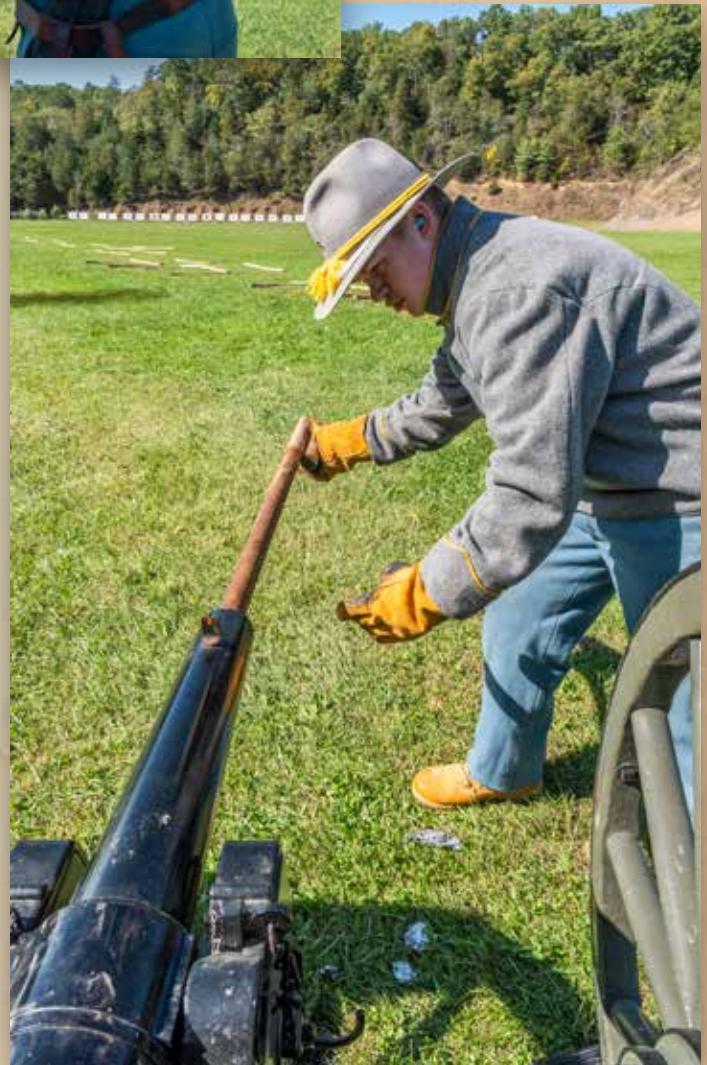
Jabin Hollinshead (position 1), Dulany Troop, 6th Virginia Cavalry, rams the projectile into Kenny Winklepleck's 3-pounder, muzzle-loading Whitworth rifle. He uses a type of safety rammer, which is designed to help protect the cannoneer in case of an accidental discharge. (Ericka Curley)
