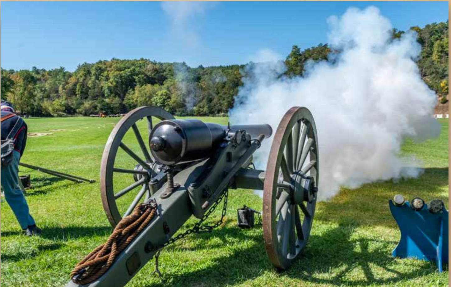
Smithgall Foundation's original, Army 20-pounder Parrott rifle, registry number 3, was manufactured at West Point Foundry in 1861, for the Commonwealth of Pennsylvania and was used by the 1st Pennsylvania Light Artillery during the Civil War. The rifling was worn because of the heavy use that the gun saw during the war, and it has a Paulson rifled liner installed to restore the bore. In the N-SSA, the 3rd U.S. Infantry competes with this impressive gun. (Ericka Curley)
